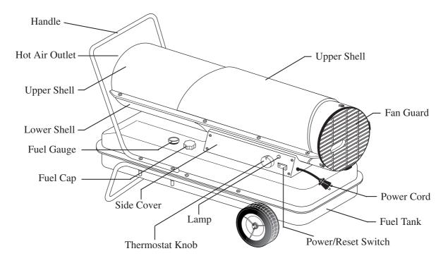
Figure 2. RMC-KFA120T / RMC-KFA170T MODELS
